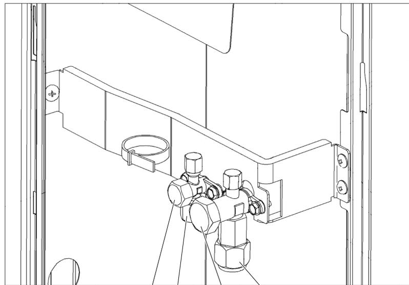
Tightening torque for valve stem cap: 19~21 N·m ④      ① Tightening torque: 68~82 N·m
